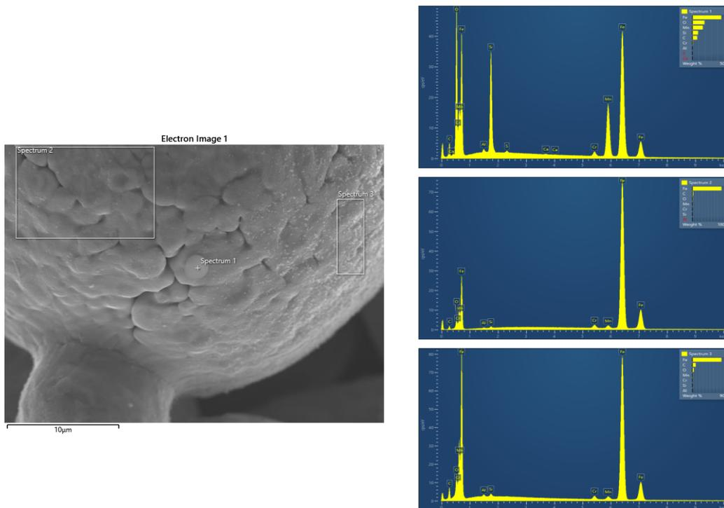
Figure 4.3 – EDS microanalyses at specific spots on surface of a powder particle
