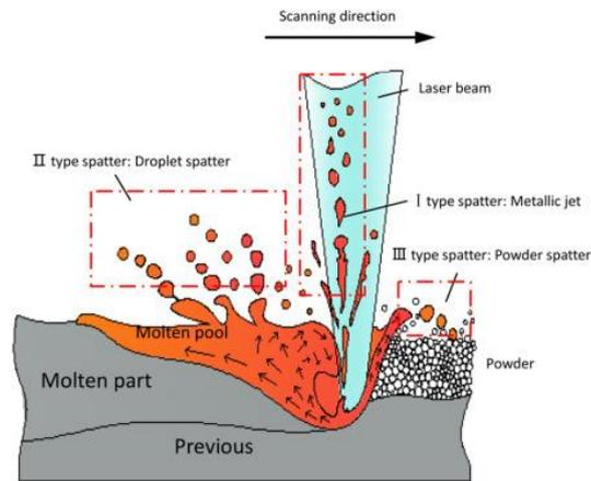
Figure 2.1 - Formation mechanisms of spatters highlighting three proposed different types of spatters [5]
