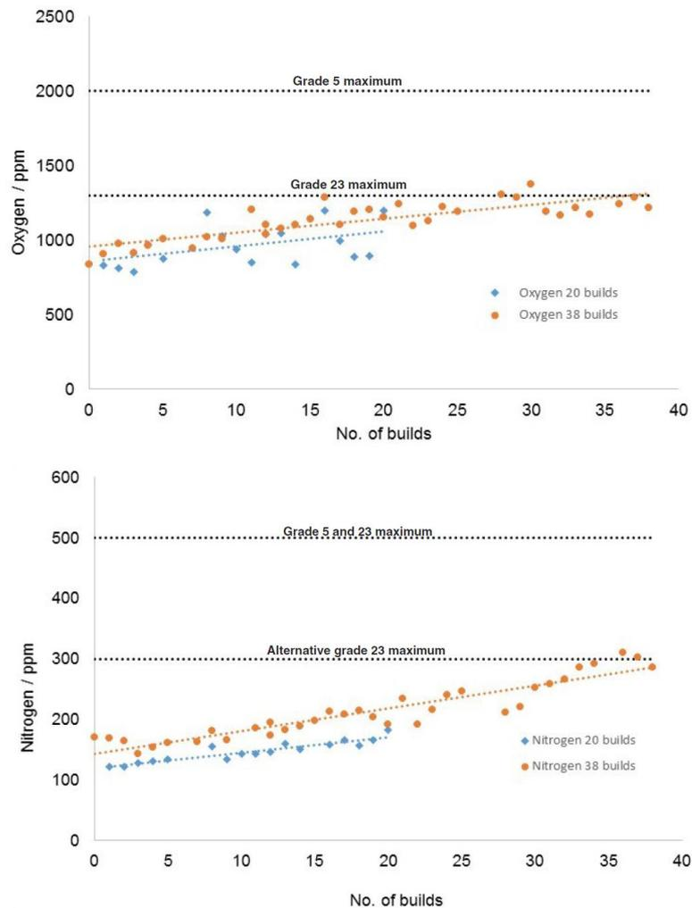
Figure 2.6 – Oxygen and nitrogen content over two separate re-use studies in a Ti-6Al-4V alloy processed by LPBF [19]
