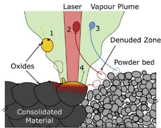
Figure 2.2 - Schematic of laser material interaction [2]
