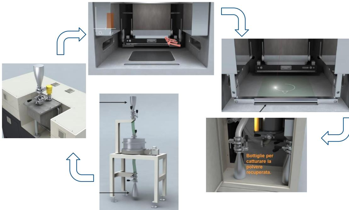
Figure 2.7 – The recycling loop of feedstock powder in LPBF [adapted from [www.renishaw.com](http://www.renishaw.com)]
