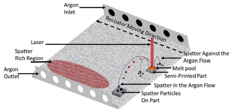
Figure 2.5 – Spatial distribution of spatters on the build plate during SLM [16]
