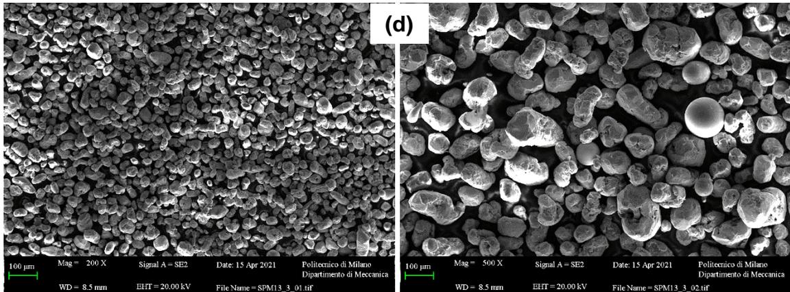
Figure 4.2 – Morphology of SPM13 powder particles as a function of the accumulated recycling runs, (a) run 0, (b) run 1, (c) run 2, (d) run 3
