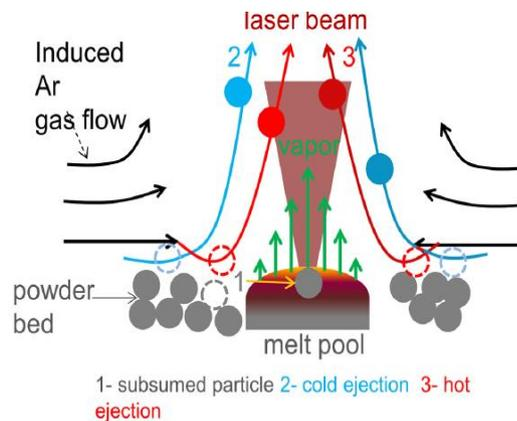
Figure 2.3 – Spatter formation mechanisms in the LPBF process [13]
