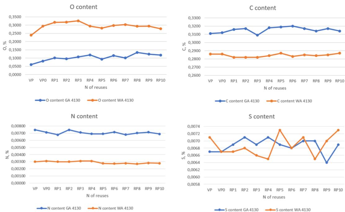
Fig. 4.1 - Chemical composition of SPM13 WA and X4130 GA steel powders after different degrees of re-use. Data taken from deliverable D4.1
