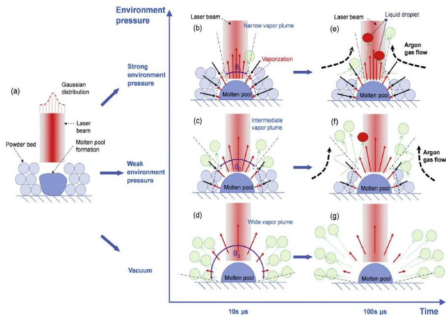
Figure 2.4 – Influence of environmental pressure in the AM system on the powder spatter behaviour [11]
