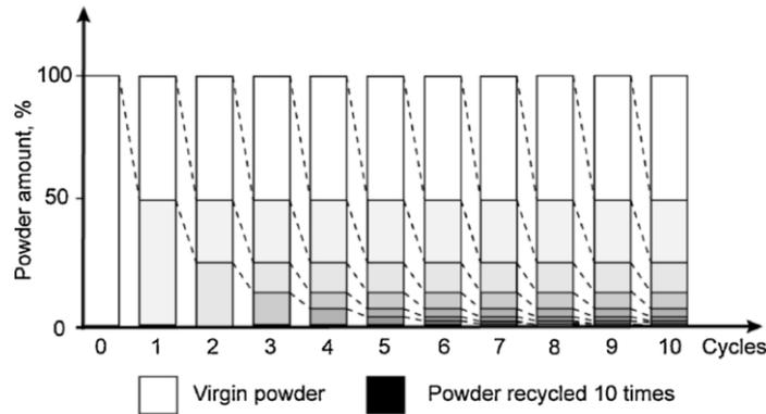
Figure 2.8 – Schematics of the recycling strategy, demonstrating the addition of 50 % virgin powder after each cycle, for 10 cycles. The greyscale indicates a continuous change of the powder state [29]
