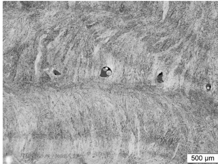
Figure 2.4 – Optical micrograph of a LMD deposit formed with the SPM11 steel showing also cavities formed at track intersections
